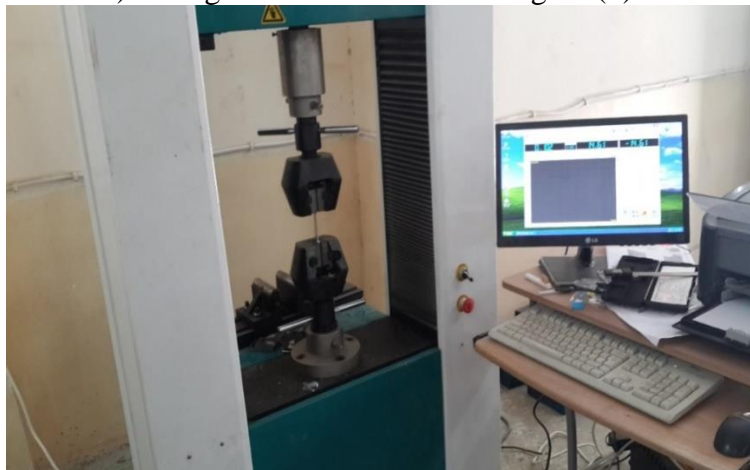
Figure (4): Tensile Test Machine (ASTM B557M – 15)
