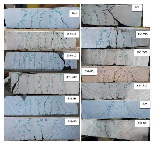
Figure (5) Beams Failure Modes and Cracking Patterns
