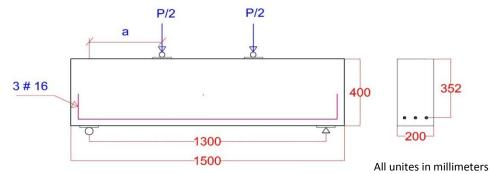
Figure (1) The Dimensions and Details of a Typical Specimen of KC Deep Beams
