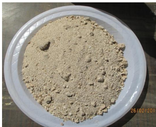
Figure (3) The gypsum after burning and before grinding.
