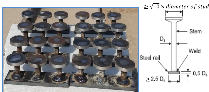
Fig. 3:- Configuration of shear studs.
