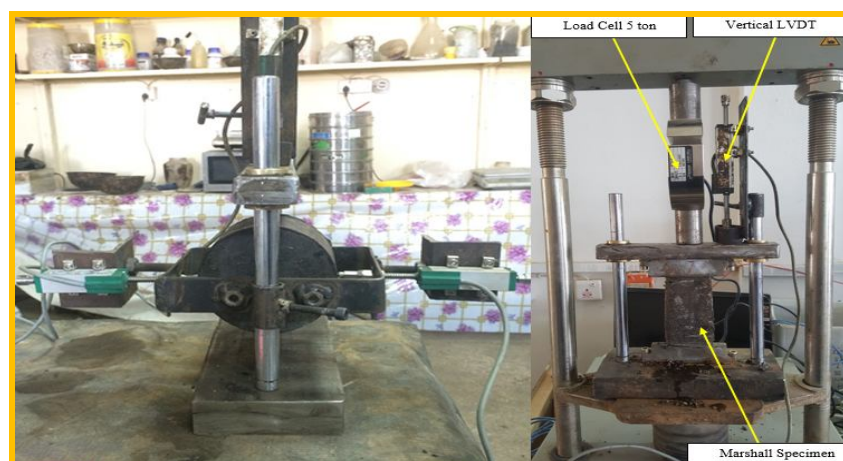
Plate 1 Indirect Tensile Strength Test Device
