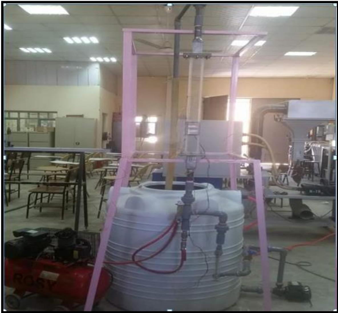
**Figure (1): The two phase flow experimental rig.**
