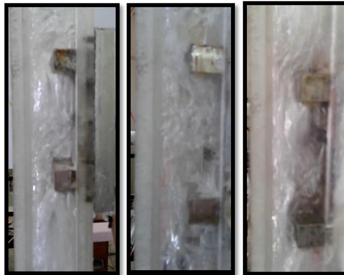
**Figure (10) : Flow image for  $g/p = 0.55, 0.73,$  and  $0.37,$  respectively at  $q = 109.65$  w**
