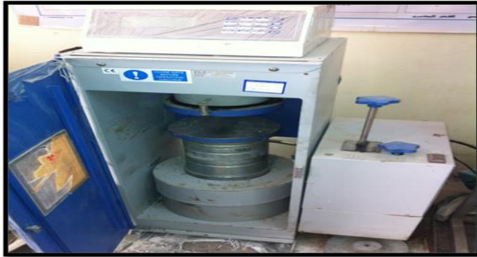
Fig.1: Compression device of concrete
