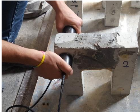
Measure UPV through old concrete piece 1 of specimen
