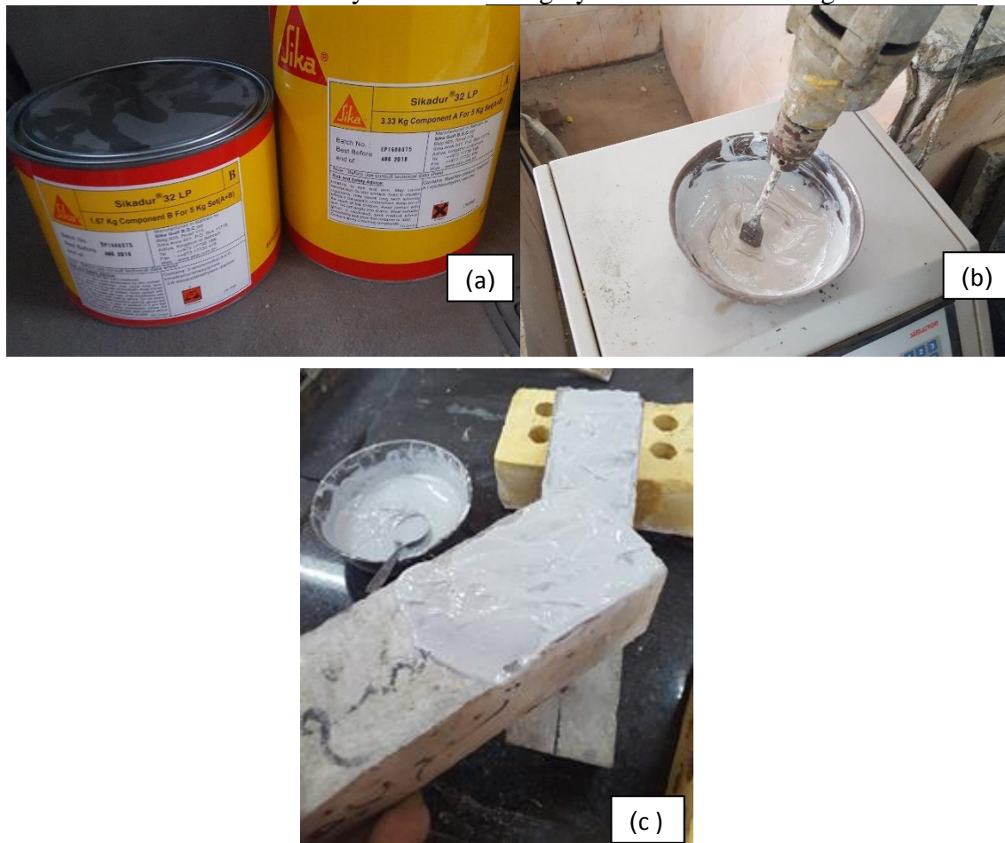
Fig. 1- Using epoxy agent between new and old concrete
