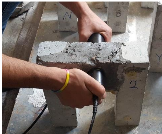
Measure UPV through new concrete of specimen
