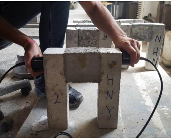
Measure UPV through old and new concrete connected together
