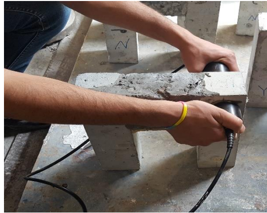
Measure UPV through old concrete piece 2 of specimen
