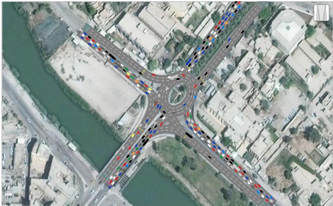
Figure 6 Output screen of PTV VISSIM simulation model of Al- Muhafadh roundabout.
