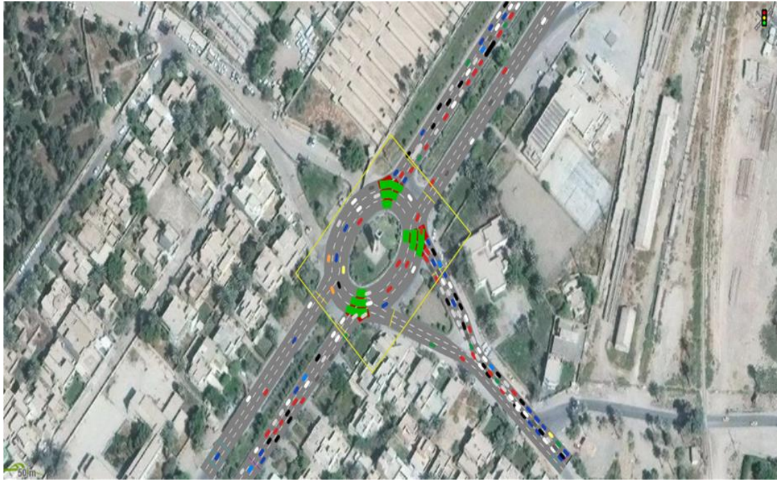
Figure 5 Output screen of PTV VISSIM simulation model of Al-Saaha roundabout.
