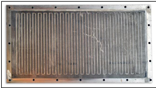
Figure (1): Test Mini-Channels Solar Collector. Figure (2): Thermocouples Location at The top Plate
