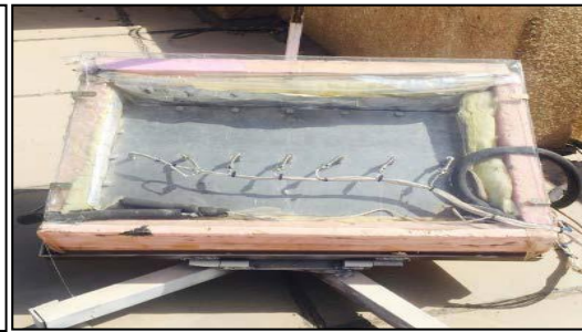
Figure (1): Test Mini-Channels Solar Collector. Figure (2): Thermocouples Location at The top Plate
