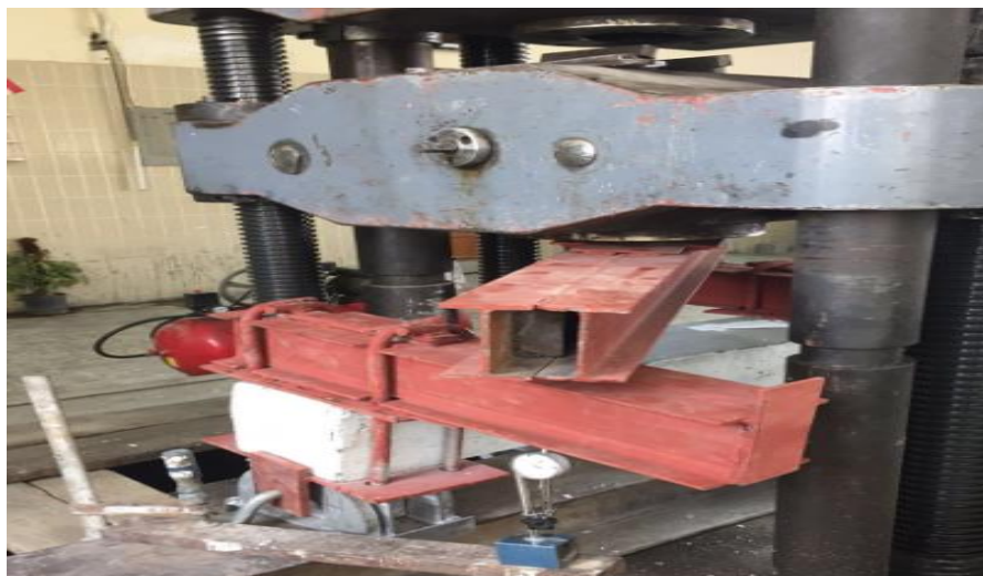
Fig. (4) Suggestions of load Arrangement Showing the Test Rig.
