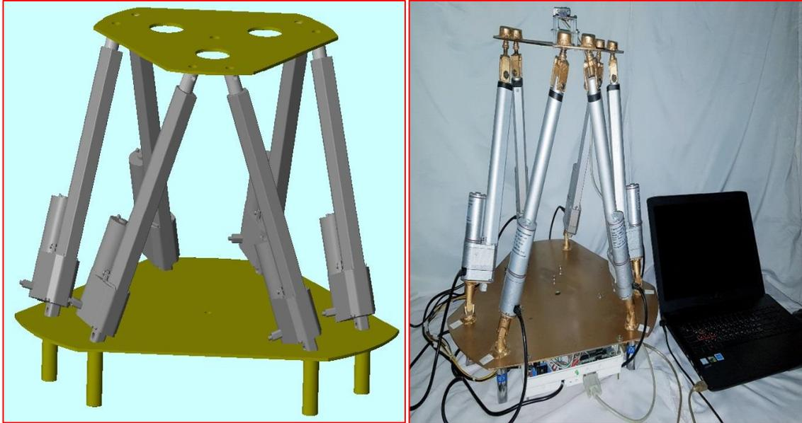
**Fig (2): The model of Gough-Stewart manipulator.**
