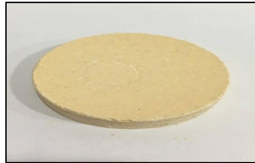
Figure (2): One of Targets after Pressing Process
