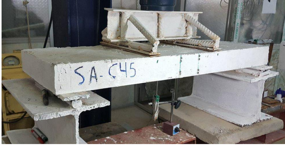
Plate 3: Loading System of the Tested Panels.
