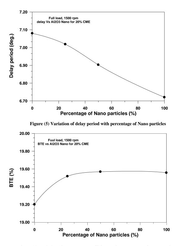
Figure (6) Variation of brake thermal efficiency with percentage of Nano particles
