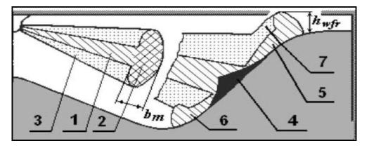
Fig. (1) Distinguishing areas of the fuel spray[17]
