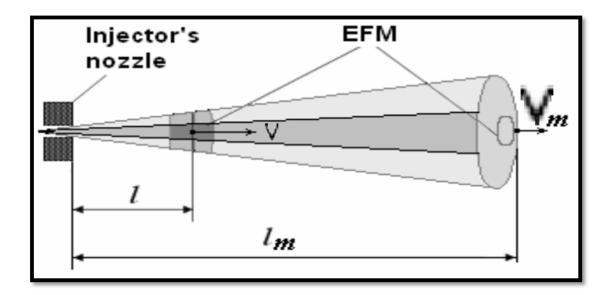
Fig. (2) Graphical shape of the fuel spray [21]
