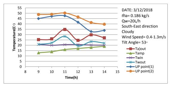
Fig. (4) Variation of Temperatures with Time for Cloudy Condition
