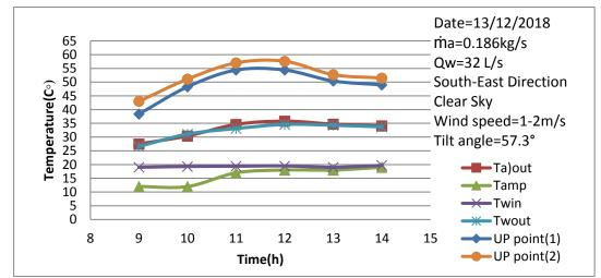
Fig. (3) Variation of Temperatures with Time for Clear Sky Condition
