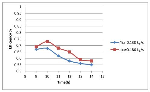
Fig (9) Effect of Mass Flow Rate on the Efficiency of the Collector
