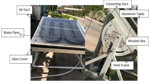
Fig. (1) The Test Rig
