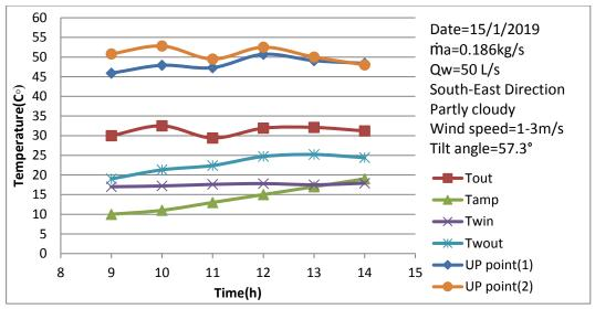
Fig. (5) Variation of Temperatures with Time for Partly Cloudy Condition
