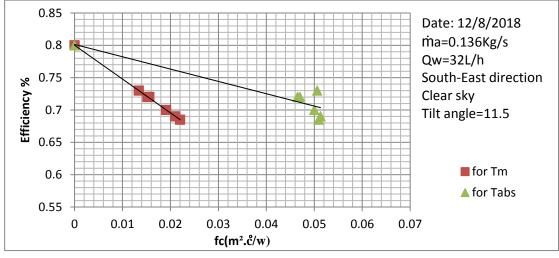
Fig (10) Performance Curve of the Collector
