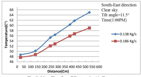
Fig (8) Mass Flow Rate Effect on the Air Temperature
