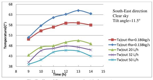
Fig (7) effect of flow rate on outlet (air & water) temperatures
