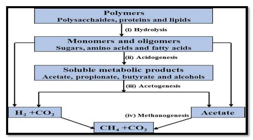
Figure 5. Anaerobicdigestion for production biogas[73].
