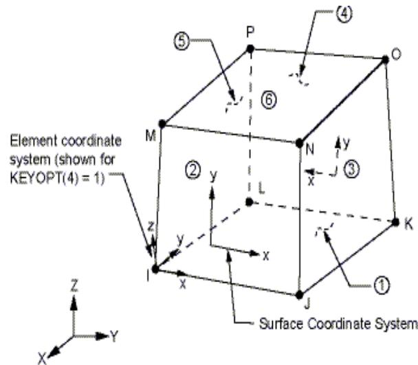
**Fig. ( 2 ) Solid45, (3-D) buried pipeline element.**
