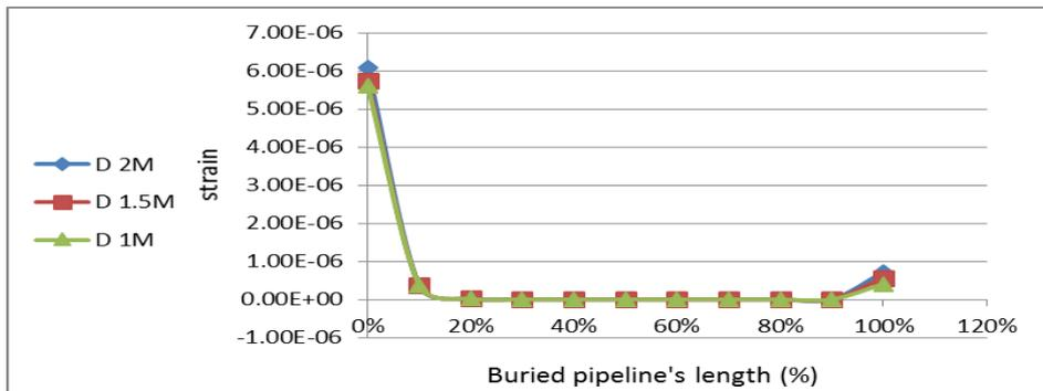
**Fig. ( 14 ) Strain–percentage of buried pipeline's length relationship for different values of depth of soil cover.**
