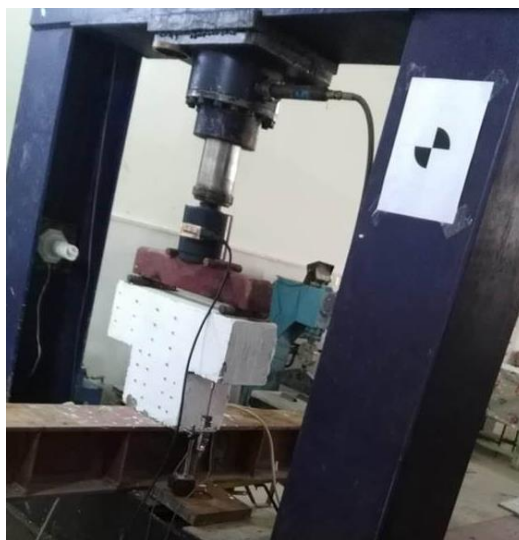
Plate 1. The Hydraulic Testing Machine of Concrete Pier Specimens
