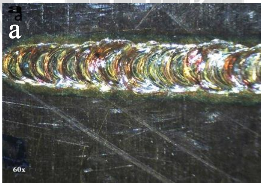
Fig 7. Pulse shapes at low magnification (a) Standard (b) Step down (c) Modulated
