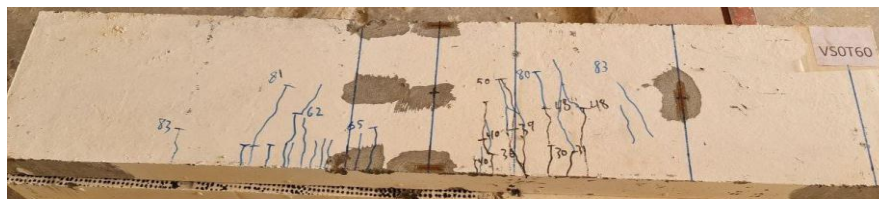
Figure 16: Cracking patterns of FEM versus experimental study for VS0T60
