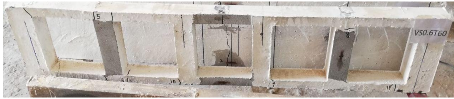
Figure 14: Cracking patterns of FEM versus experimental study for VS0.6T60
