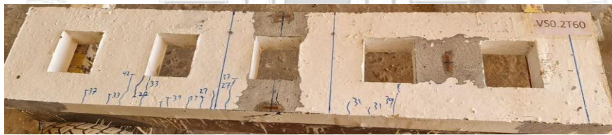
Figure 15: Cracking patterns of FEM versus experimental study for VS0.2T60
