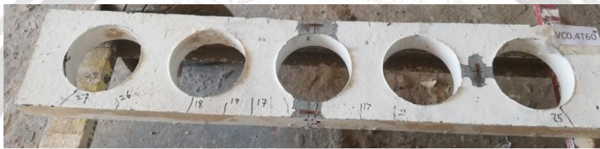
Figure 12: Cracking patterns of FEM versus experimental study for VC0.4T60
