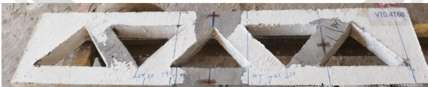
Figure 13: Cracking patterns of FEM versus experimental study for VT0.4T60
