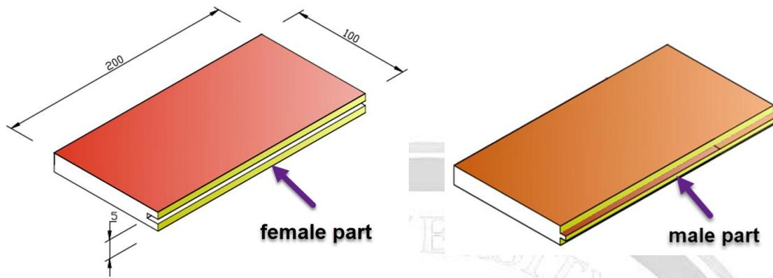
Figure 1: Welding Specimens with Male and Female Sides (dimensions in mm)
