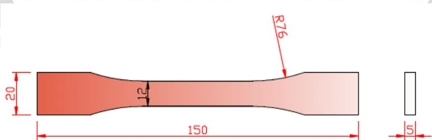
Figure 6: Tensile Test Specimen with ASTM D638-03
