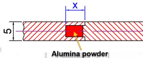
**Figure 5: Assembly of the Two Parts of the Welding Specimen**
