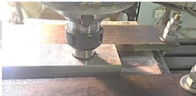
Figure 3: Illustration of the FSW tool during the welding process
