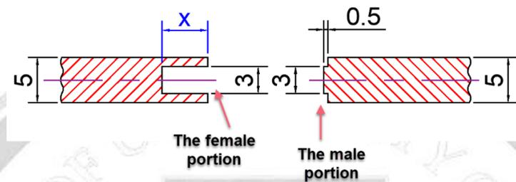
**Figure 4: Preparation of the Two Parts of the Welding Specimens (dimensions in mm)**
