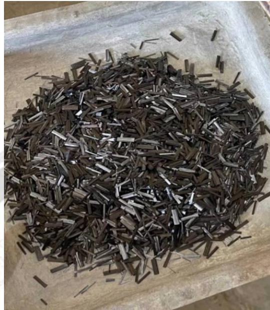
Figure 2: Carbon Fiber Used to produce The ECC Specimens.
