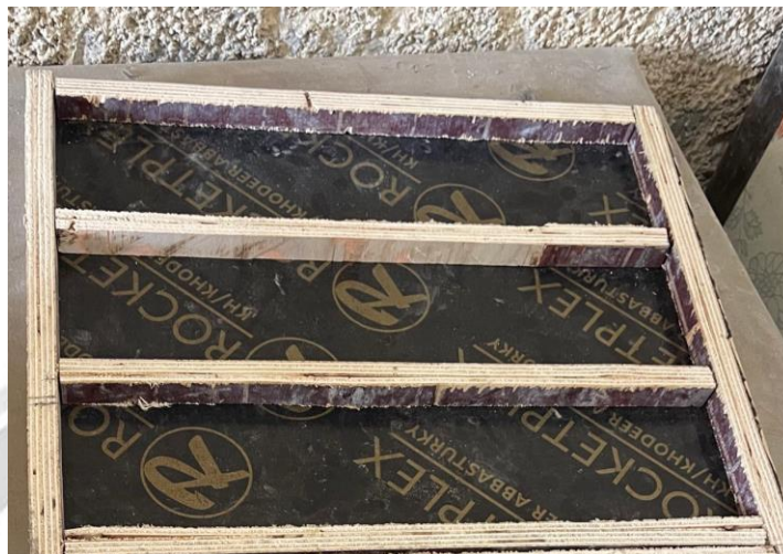
Figure 3: Beam Mould (Length 400mm, Width 100mm, Thickness 2cm)
