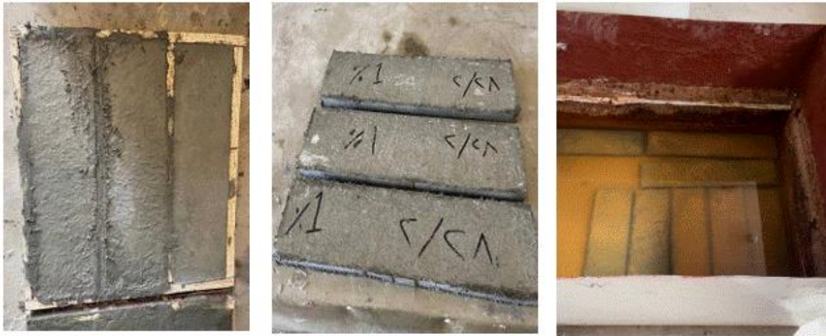
Figure 5: Specimens Casting and Curing.
