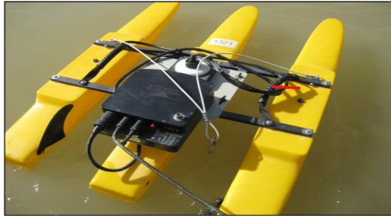
Fig. 2: SonTek river surveyor ADCP [12].
