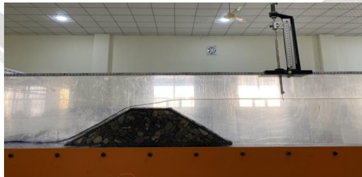
Figure (3) Trapezoidal Gabion weir during experiment
