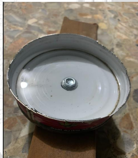
Fig. 21 Pod is mounted to frame with self-drill bolt
