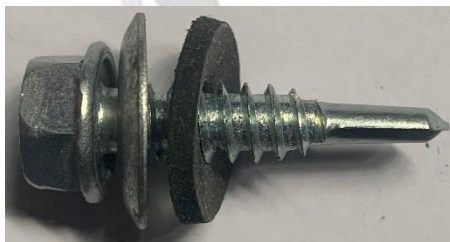
a- Seal is separated from Washer
