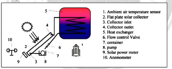
Fig. 1. The experimental set up schematic [11]
