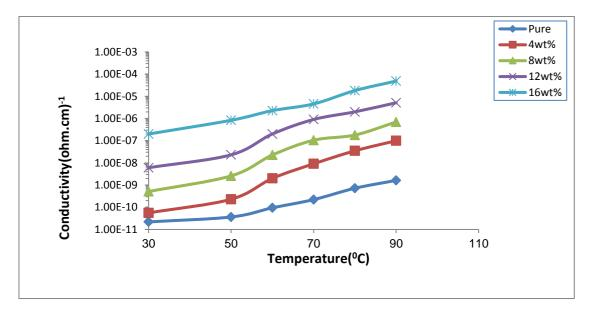
Figure 3: Variation of D.C. electrical conductivity with temperature for (PVA- $Al_2O_3$ )nanocomposites
