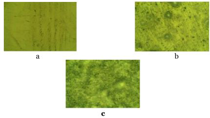
"Figure 2: Photomicrographs for PVA-Al<sub>2</sub>O<sub>3</sub>nanocomposites (a) for pure,(x320). (b) for 4wt.% Al<sub>2</sub>O<sub>3</sub> ,(x320). (c) for 16wt.%Al<sub>2</sub>O<sub>3</sub> ,(x320).
