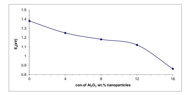
Figure 5: Variation activation energy for D.C. electrical conductivity with Al<sub>2</sub>O<sub>3</sub>wt.% concentration for (PVA-Al<sub>2</sub>O<sub>3</sub>) nanocomposites.
