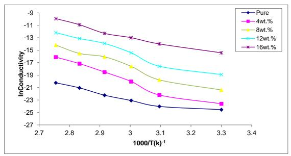
Figure 4: Variation of D.C. electrical conductivity with reciprocal absourcemperature for (PVA-Al<sub>2</sub>O<sub>3</sub>) nanocomposites.
