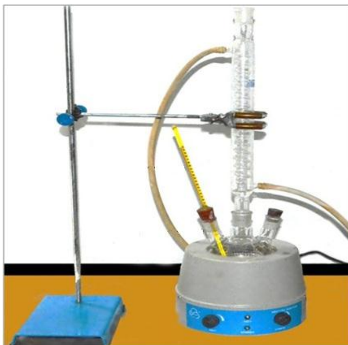
Figure : The leaching cell
