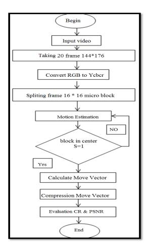
Fig4: The Block Diagram Source Coding Algorithm
