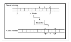
Fig 2. Code Structure of General Convolutional Codes.
