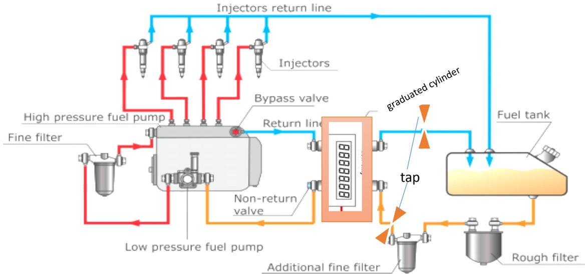
**Fig .1. Fuel consumption measurement device by graduated cylinder**
