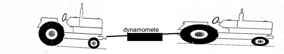
Fig .1. dynamometer connecting between two machines (MF-440 Exrta and MF-265s )
