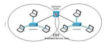
Figure 1.3 ESS WLAN
