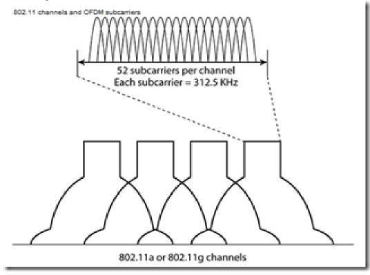
Figure 1.8 802.11 Channel and OFDM subcarriers
