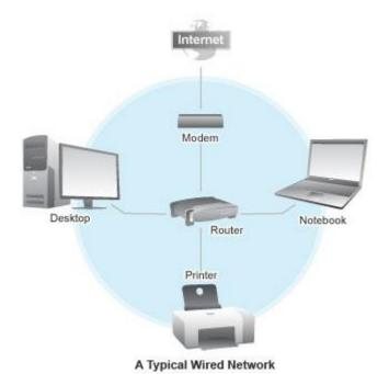
Figure 1.4 wired network components
