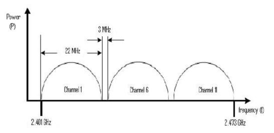
Figure 1.7 DSSS non overlapping channels
